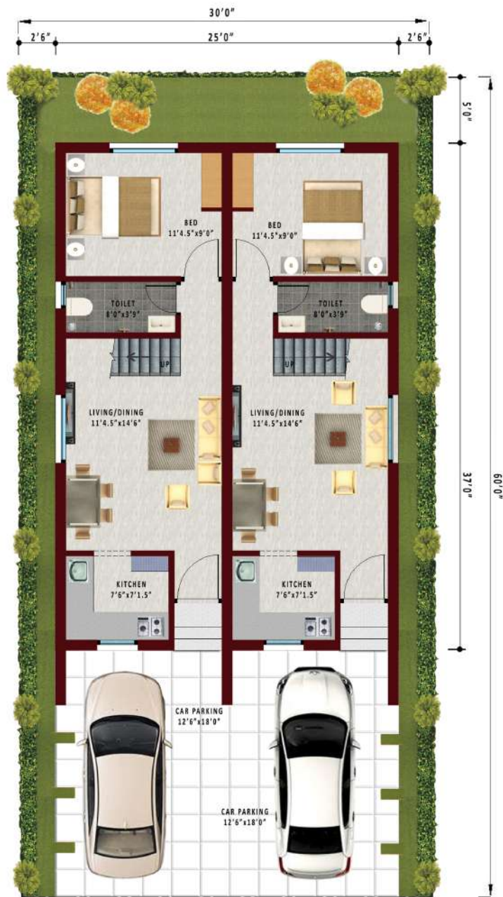
SITE CUM GROUND FLOOR PLAN
