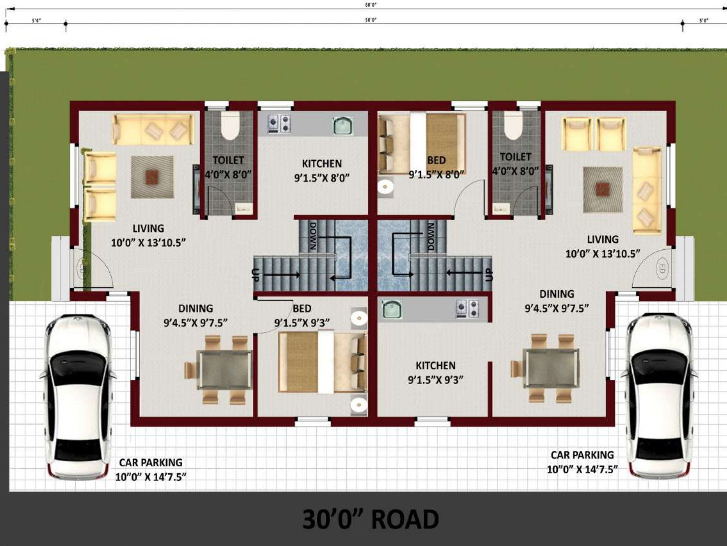
SITE CUM GROUND FLOOR PLAN
