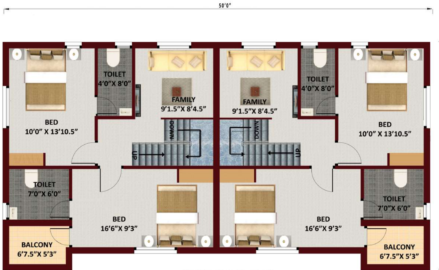
FIRST FLOOR PLAN
